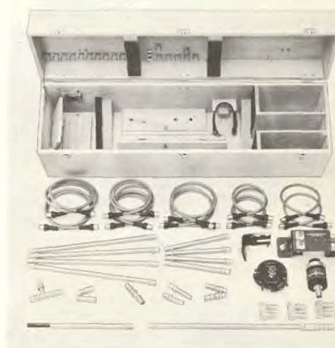
Figure 23. View of the instrument storage box with accessories that are supplied with the Type 1607-A Transfer-Function and Imittance Bridge.
